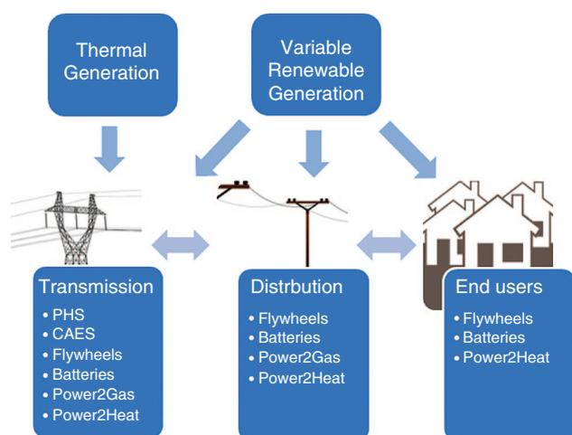
Figure 3.1 Storage technologies in EU electricity grids.
