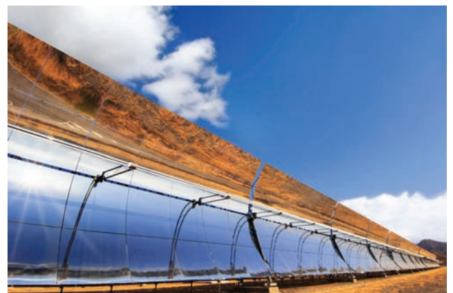
Figure 3.5 Solar receiver for trough technology (DLR, Markus Steur).
